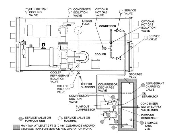
Fig. 20 — Optional Pumpout System Piping Schematic with Storage Tank
